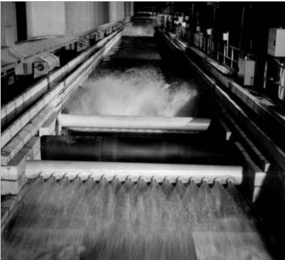
Pretreatment in a pickling line
